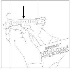
2. Bend end of band toward underside to form a 1"-2" hook and insert in band slot of housing. Wrap the assembly snugly around object and at a point TWO INCHES BEYOND first serration, cut, then bend a second 1"-2" hook toward underside of band.
