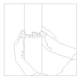
3. Insert hook into either band slot on both housing and rack and flatten with thumb, forming clamp. Tighten screw with screwdriver to desired tension. Clamp is complete.
