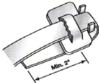
2. Holding the buckle in one hand, with ears pointing upward and to the right as shown, insert the band through the buckle "bridge", past the ears and bend so that at least 2 inches are underneath the buckle.
