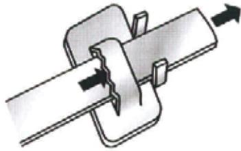
1. Pull appropriate length of band from BAND-IT tote (approx. 3-1/2 times the diameter of the pole or mastarm for a single-wrapped clamp and seven times the diameter for a double-wrapped clamp. Add 6-8 inches for both single-wrapped and double-wrapped clamps to accommodate the tail and bracket design.) Cut the band using one of the BAND-IT tools with built-in cutter.
