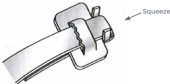
3. Squeeze this "buckle wrap" to flatten the bend preventing "pull-out" during tensioning
