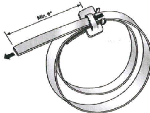
5. Repeat a second wrap of band through the bracket and buckle for a continuous double-wrap application. Double-wrapping develops greater clamp tightness than single-wrapping clamps and more than doubles the holding strength for heavy objects and high wind loads.
