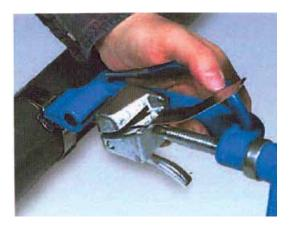
7. To set the lock and cut off band, roll tool nose over buckle, relieving a slight amount of tension by backing off tension handle **during** this fold over operation. Failure to back off tension handle throughout the entire course of roll over may result in breaking band. On the other hand, releasing too much tension may result in a loose clamp. We suggest 1/2 to 1 full turn of the spin handle during release.
