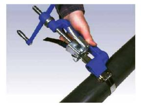
6. Place band in open slot of tool nose and gripper block. Move into slot as far as possible to prevent buckle from sliding into tool nose. With thumb on band gripper lever, apply tension by turning handle of tool. After tension is created, it is no longer necessary to hold the band gripper lever as it locks itself under tension. When band stops moving through buckle, maximum tension has been applied. Stop turning handle.
