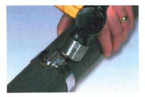
9. Remove tool, holding stub of band down with thumb.
