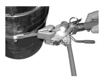
1. With the Bantam Tool in the Straight Position, place the band in the tool with sufficient band in the winding mandrel.
