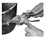
2. With ratcheting action, tension the band until clamp is tight.
