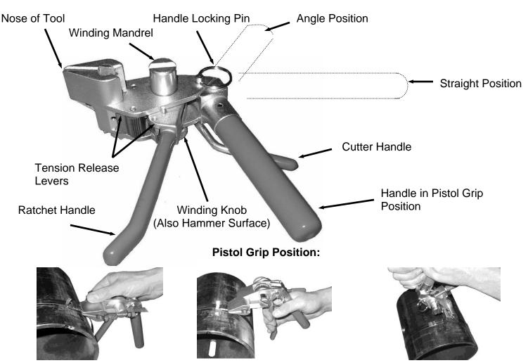
1. With the Bantam Tool in the Pistol Grip Position, place the band in the tool with sufficient band in the winding mandrel.
