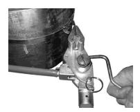
3. Roll tool over as far as tool will go, and push forward cutter handle. Remove tool and tap down ears of clip to complete clamp.
