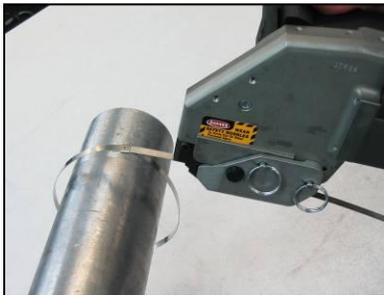
2. Begin tensioning clamp by pushing and holding down operating trigger
