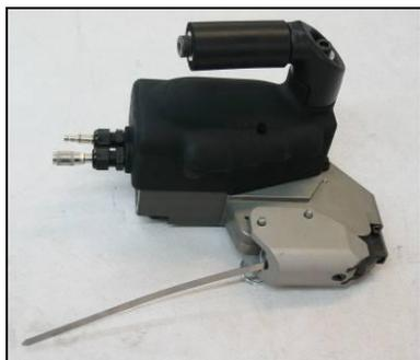
5. After clamp is completed, clamp tail scrap must be removed from tool. Clamp tail scrap is not ejected automatically. Tool is now ready for next clamp.
