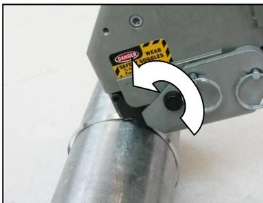
4. While tensioning clamp, hold tool slightly tipped forward. This will assist proper clamp installation. Continue to hold down operating trigger until tool completely tensions and cuts off clamp. Release trigger after cut off.
