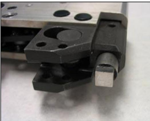
Once the pin is removed, grasp the Knife Assembly with a pair of needle-nose pliers and pull out of tool head. Examine for wear and replace if needed.
