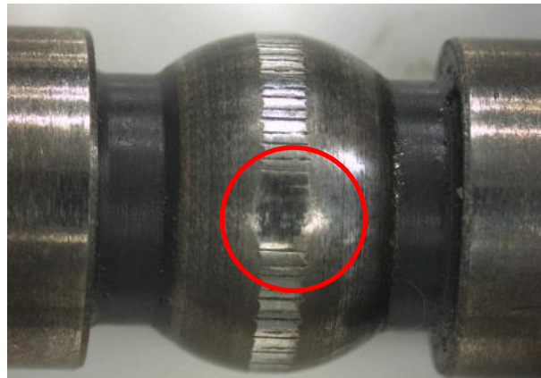
A worn out tension gripper: Ridges are worn off in some sections
