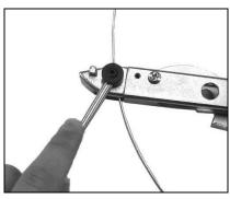
1. Cut off adequate band from roll of 1/4" or 3/8" BAND-IT band by opening the slot in the head of the tool with the cut off lever at right angles to the tool. Thread the band through the slot and cut.
