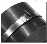
7. Insert tail of the preformed BAND-IT Jr. clamp into the tool. Tension as shown in steps 2 & 3. When tensioned sufficiently, release locking pawl and rotate over object being clamped. Cut off, leaving stub.
