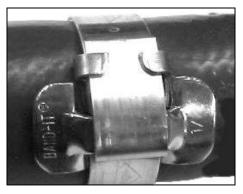
**5.** Complete clamping operation by tapping down ears of buckle with a hammer or mallet.
