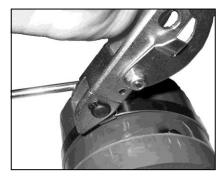
**8.** This stub should be shortened. With cutter in the open position, Place tool over stub, insert into slot and trim off excess.
