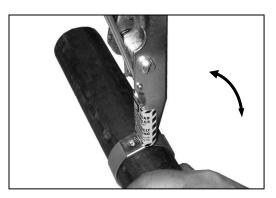
**4.** Still holding tension with wrench, pivot tool up against buckle, then backward several times to break off clamp tail.
