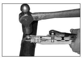
**3.** Place punch on clamp and, while holding tension with ratchet wrench, lock clamp by striking punch at least once. Varying blows may be required depending on object being clamped.
