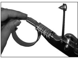
1. Tool is designed specifically for 3/8" and 5/8" center punch clamps only. Insert clamp in tool's appropriate slot and insert wrench assembly. If you prefer, install wrench assembly before clamp is inserted. Slot must be aligned with clamp tail.
