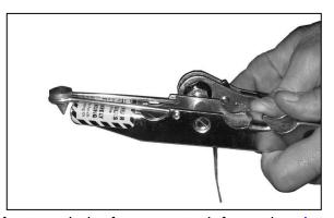
**5.** To loosen clamp tail, wind ratchet wrench until tail is free. Remove ratchet wrench assembly and clamp tail. Caution: Clamp tail may spring back once released from tool nose.
