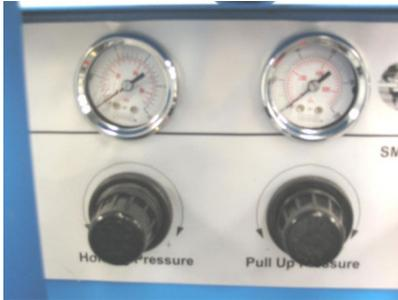
Air pressure setting can be made using the regulators and gauges on face of the tool.
