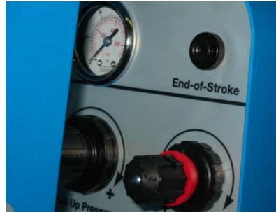
End-of-Stroke Indicates the desired clamp tension and cut-off has not occurred. Also shown is speed control with red lock ring.
