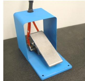
Dual function foot control valve. Pressing forward activates clamp installation. Heel action activates tail return and prepares for next clamp.
