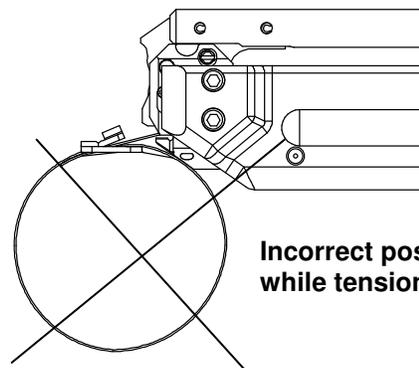
**Incorrect position of tool while tensioning**
