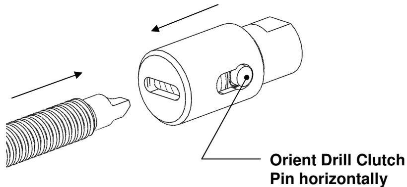
**NOTE: Alignment is critical for proper tool function.**
