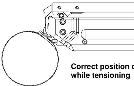
**Correct position of tool while tensioning**
