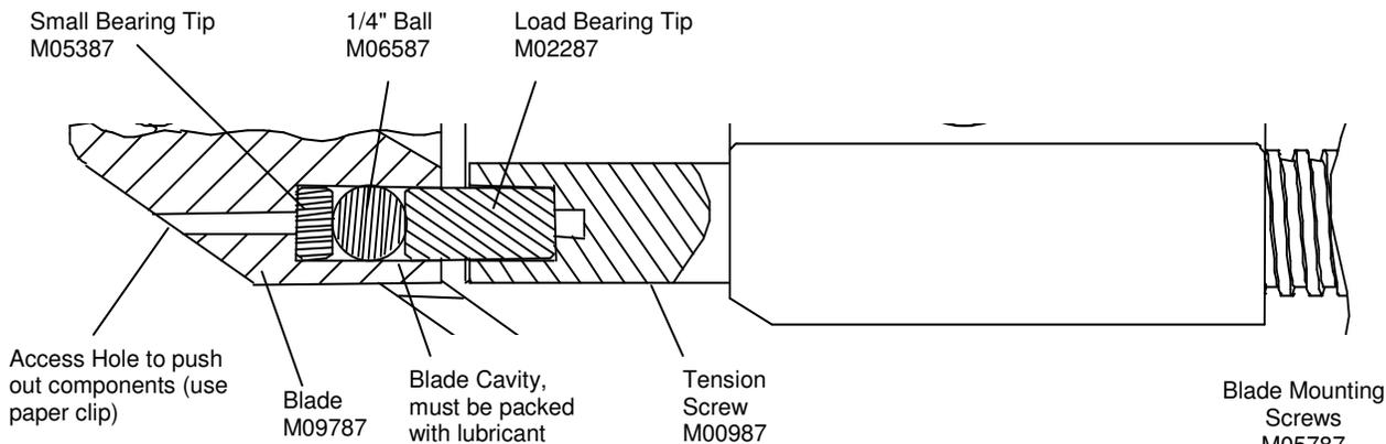
3. To gain access to bearing components: remove blade Mounting Screws (2 places) and slide Blade free. Paper clip may be used to push bearing components out of Blade. Wipe lubricant from components. If ball or bearing tips appears heavily worn, replace with new one. Note: 1/4" ball is made from hard tungsten carbide material, do not replace with regular ball bearing. (Smooth indentation from ball in the bearing tips is normal).
