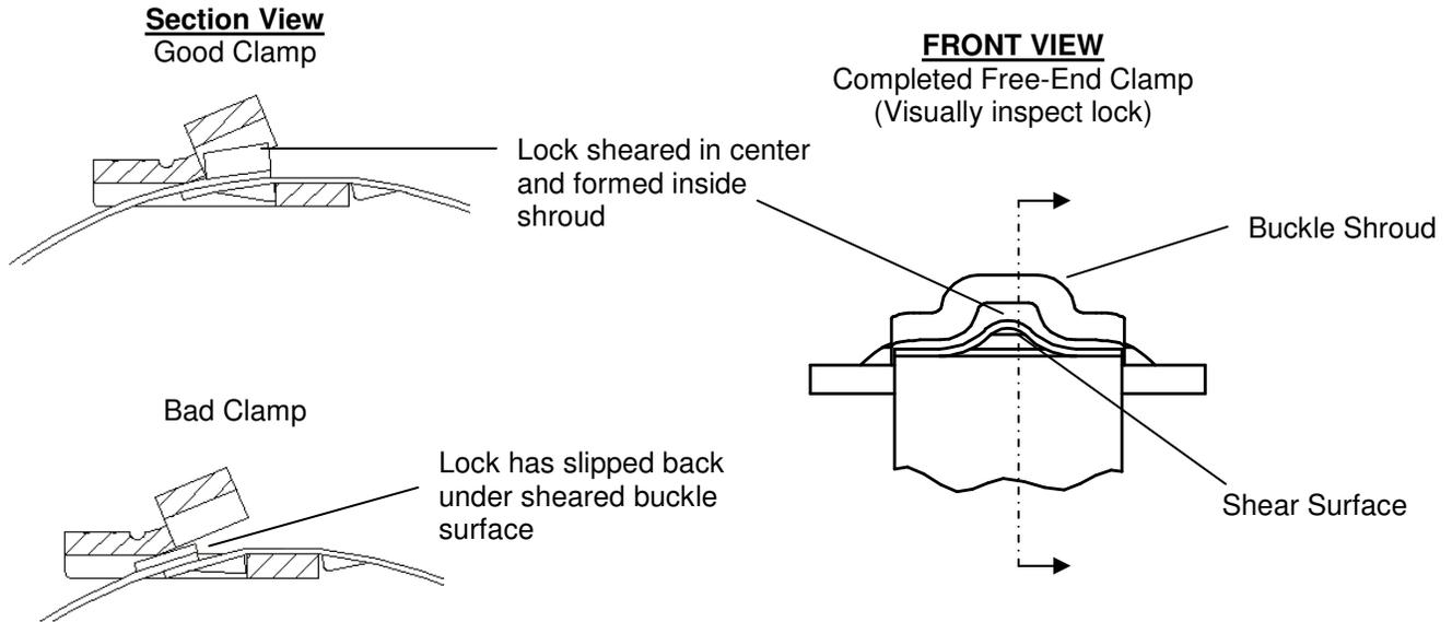
**Important:** Visually inspect lock formed in band as shown. If lock has slipped under the sheared surface of the buckle, remove clamp and install a new one at reduced tension by lowering the Drill Clutch torque setting.
