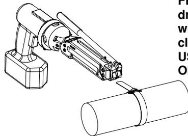
**DO NOT FEATHER the drill's TRIGGER when tensioning a clamp. USE FULL SPEED OF TOOL**
