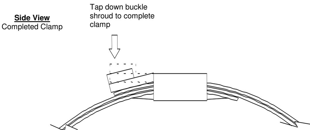
When applying clamps on soft, thick-walled hose, tension clamp then wait a full 30 seconds. Clamps may be re-tensioned by squeezing the Drill Switch on the power unit a second time prior to forming the lock and cutting the excess clamp tail. This allows hose to “settle” under the band of the clamp. This hose material attribute is called Cold Flow. Finally, complete clamp by tapping down the buckle shroud as described above.
