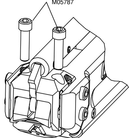
5. To replace Gripper: Make sure Tension Block is all the way forward against the tool head. Remove drill. Remove tool adapter body. Remove one side of the tool body or the other, not both. Slide Gripper out sideways and replace with a new one. Re-attach Tool Body side. **Caution:** Do not push or move Tension Block while Gripper is out of tool.
