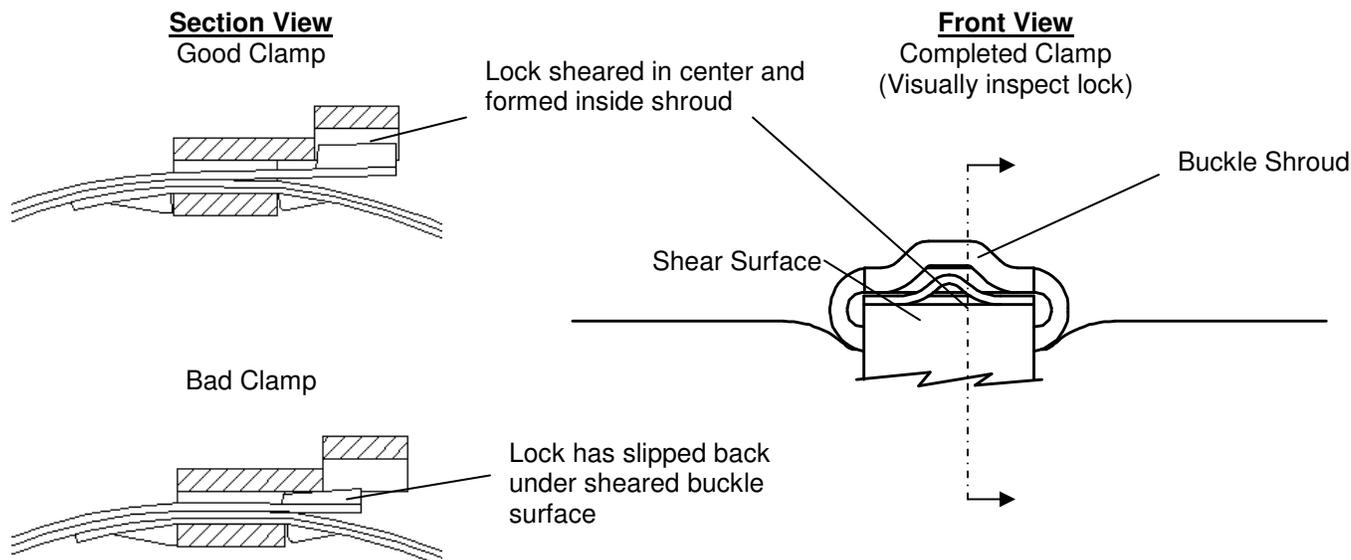
**Important:** Visually inspect lock formed in band as shown. If lock has slipped under the sheared surface of the buckle, remove clamp and install a new one at reduced tension by lowering the Drill Clutch torque setting.
