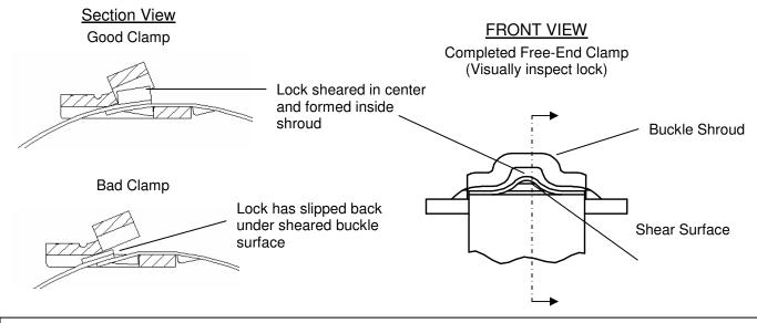
Important: Visually inspect lock formed in band as shown. If lock has slipped under the sheared surface of the buckle, remove clamp and install a new one at reduced tension by lowering the drill clutch torgue setting.
