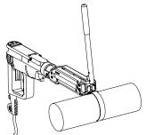
has been applied. Lift the cut-off handle to cut tail off and form a lock. Excess band can be removed by pulling out from rear of tool or reversing the drill.
